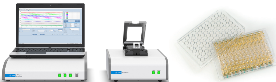
Figure 1. The Agilent xCELLigence RTCA Cardio instrument. The RTCA Cardio instrument is a label-free, real-time system that monitors cardiomyocyte beating and cell viability for assessment of cardiac toxicity. It is composed of the RTCA Cardio control unit, the RTCA Cardio analyzer, the RTCA Cardio station (placed in a CO 2 incubator), and the E-Plate Cardio 96 or E-Plate Cardio VIEW 96, which contains interdigitated gold biosensors fabricated in the bottom of each well.
