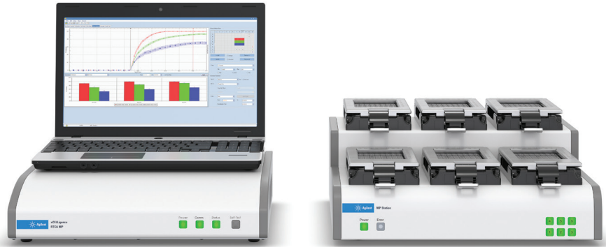
Figure 1A. The Agilent xCELLigence RTCA MP instrument monitors cell proliferation, morphology change, and attachment quality in a label-free, real-time manner. The MP (multiple plate) model can host up to six 96-well E-Plates. The instrument is placed in a standard CO 2 cell culture incubator and interfaces via a cable with analysis and control units that are housed outside the incubator.
