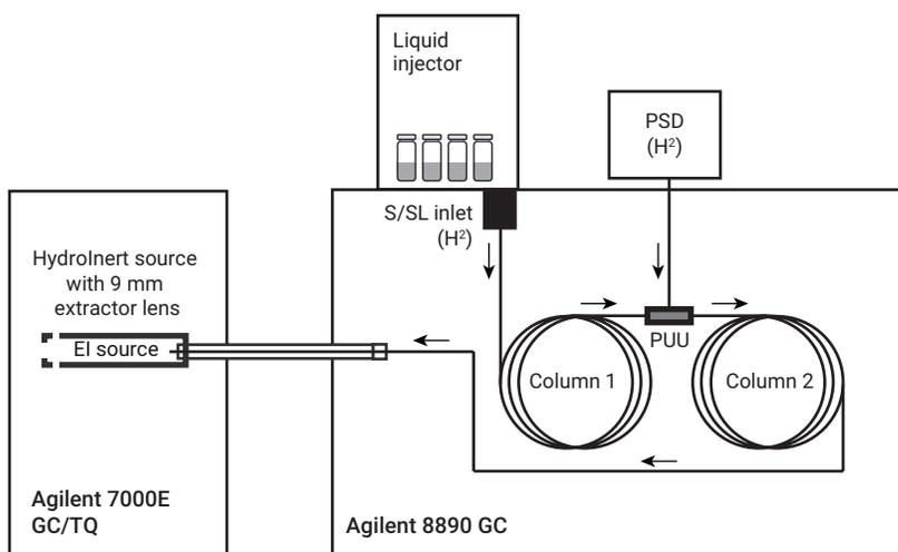
Figure 1. System configuration.
