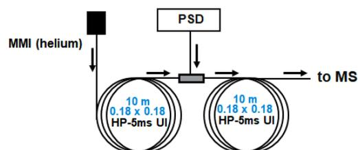
Figure 1. The Agilent GC/TQ system featuring two utilized midcolumn backflush configurations (right).
