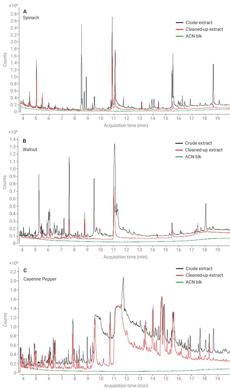
**Figure 4.** Scan TIC of the spinach (A), walnut (B), and cayenne pepper (C) extracts. The red trace corresponds to matrix sample with Captiva EMR cleanup, and the black trace corresponds to matrix sample without clean up. The green trace corresponds to the acetonitrile solvent blank.
