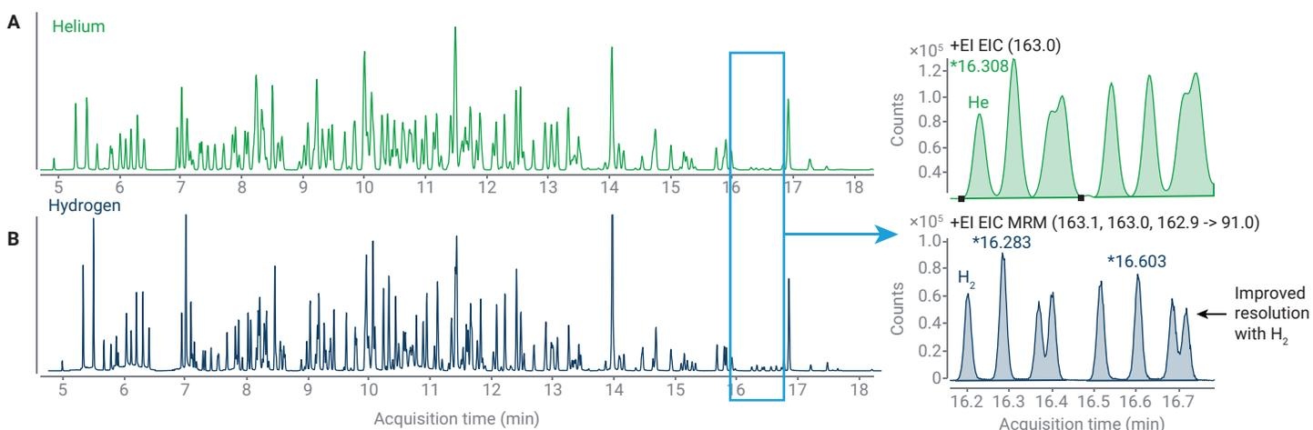
**Figure 3.** MRM chromatograms for a mixture of (A) 203 pesticides acquired with helium carrier gas with the conventional 20-minute method, (B) 203 pesticides acquired with hydrogen with the 20-minute method using a 20 m × 20 m minibore configuration.
