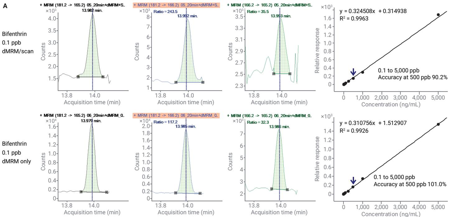
**Figure 8A.** Quantifier and qualifier ion profiles and matrix-matched calibration curves over 0.1 to 5,000 ppb for bifenthrin spiked at 100 ppb in cayenne pepper with the Agilent 7000E GC/TQ in simultaneous dMRM/scan and dMRM only data acquisition modes.
