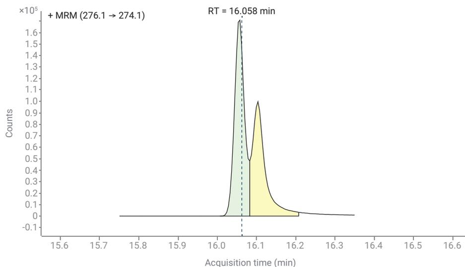
**Figure 2.** Indeno[1,2,3-cd]pyrene and dibenz[a,h]anthracene at 2.0  $\mu\text{g}/\text{mL}$  (62.6% resolution).
