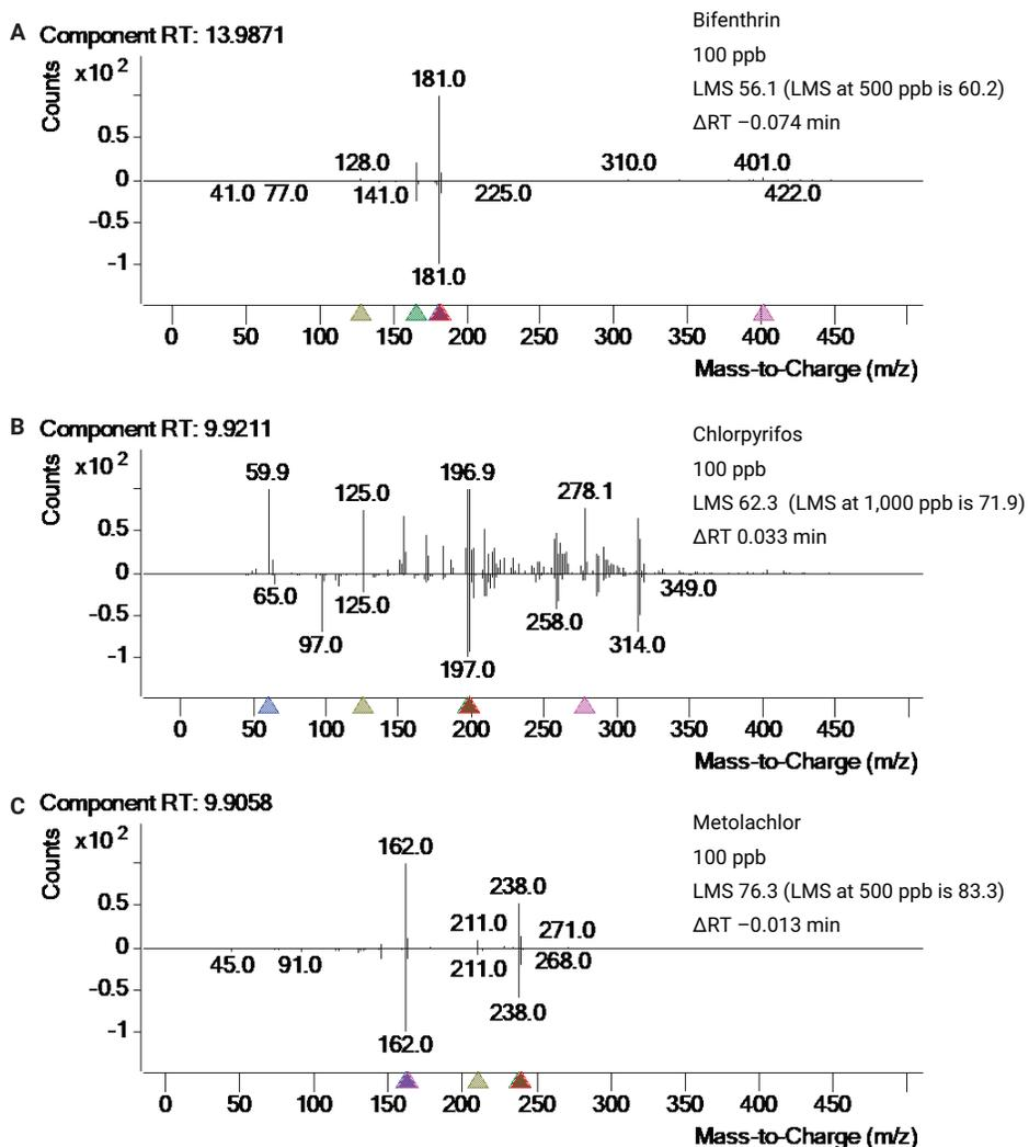
**Figure 7.** Spectral confirmation with library match score for bifenthrin (A), chlorpyrifos (B), and metolachlor (C) spiked at 100 ppb in cayenne pepper with the Agilent 7000E GC/TQ in simultaneous dMRM/scan data acquisition mode.
