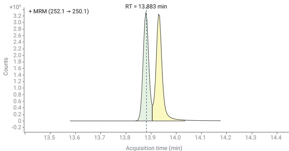
**Figure 1.** Benzo(b)fluoranthene and benzo(k)fluoranthene at 2.0 µg/mL (88.6% resolution).
