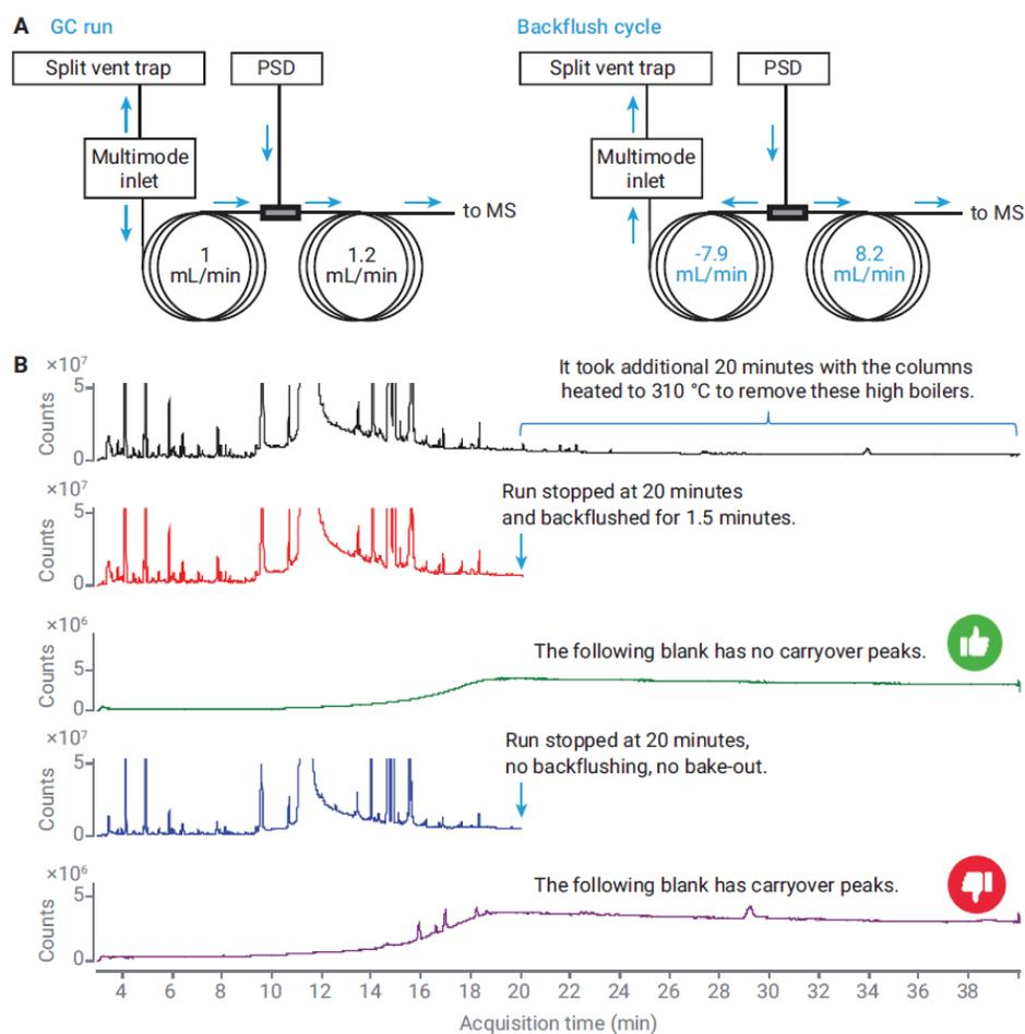
**Figure 5.** Midcolumn backflush configuration and gas flow during the GC run and the backflush cycle (A); TIC Scan chromatograms of a cayenne pepper extract followed by the analysis of an instrument blank with column bake-out, with backflush and without backflush or bake-out (B).
