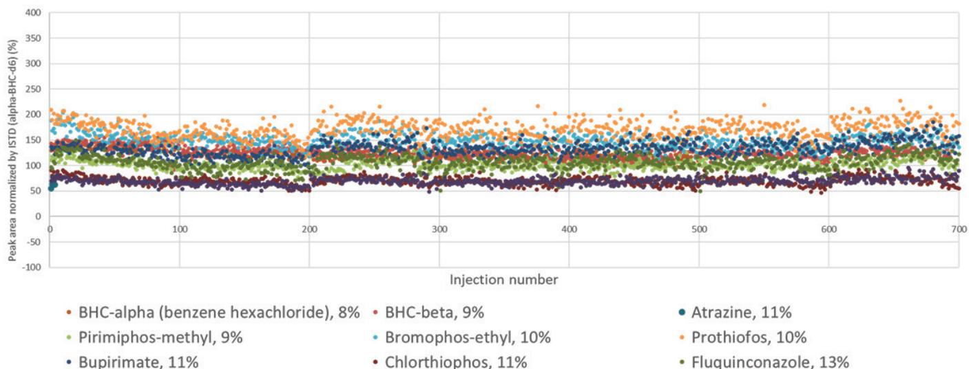
**Figure 7.** Stability of the peak area for pesticides spiked at 20 ppb into spinach extract, normalized by the ISTD, over 700 consecutive injections. The 10-minute analysis using the conventional 15 × 15 m column configuration coupled with the Agilent 7000E triple quadrupole GC/MS.
