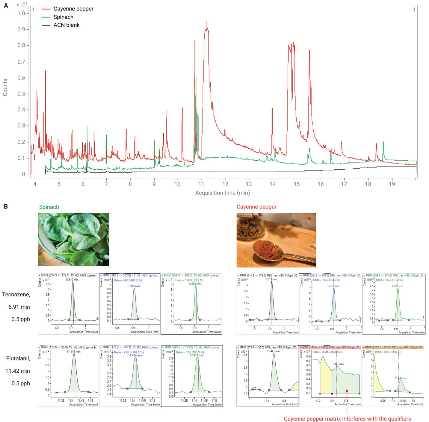
**Figure 9.** Scan total ion chromatogram (TIC) of the spinach and cayenne pepper QuEChERS extracts, and acetonitrile blank (A). MRM chromatograms for tecnazene and flutolanil in spinach and cayenne pepper extracts at 0.5 ppb acquired with the Agilent 7010C GC/TQ with hydrogen carrier gas (B).
