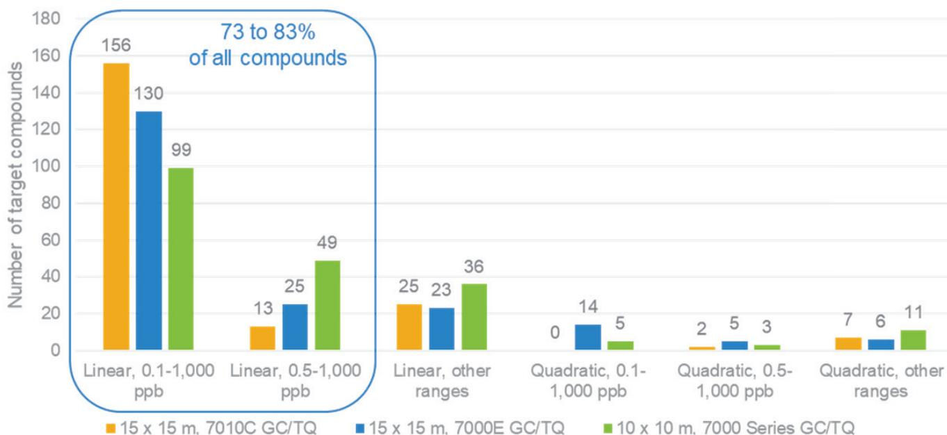
**Figure 6.** Calibration performance for the 203 pesticides with the 10-minute methods using the conventional 15 × 15 m configuration, coupled with the Agilent 7010C and 7000E triple quadrupole GC/MS systems, and the minibore 10 × 10 m configuration, coupled with the Agilent 7000 series triple quadrupole GC/MS in spinach. The graph shows the number of compounds and their calibration ranges.
