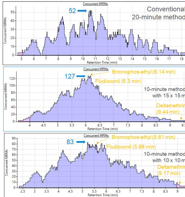
**Figure 2.** The distribution of 614 dMRM transitions with the 20-minute conventional pesticide analysis, the 10-minute analysis employing the conventional 15 × 15 m configuration, and the 10-minute method employing the minibore 10 × 10 m column configuration.
