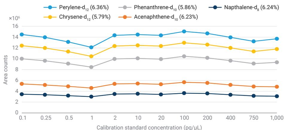
Figure 3. ISTD response over the calibration range.
