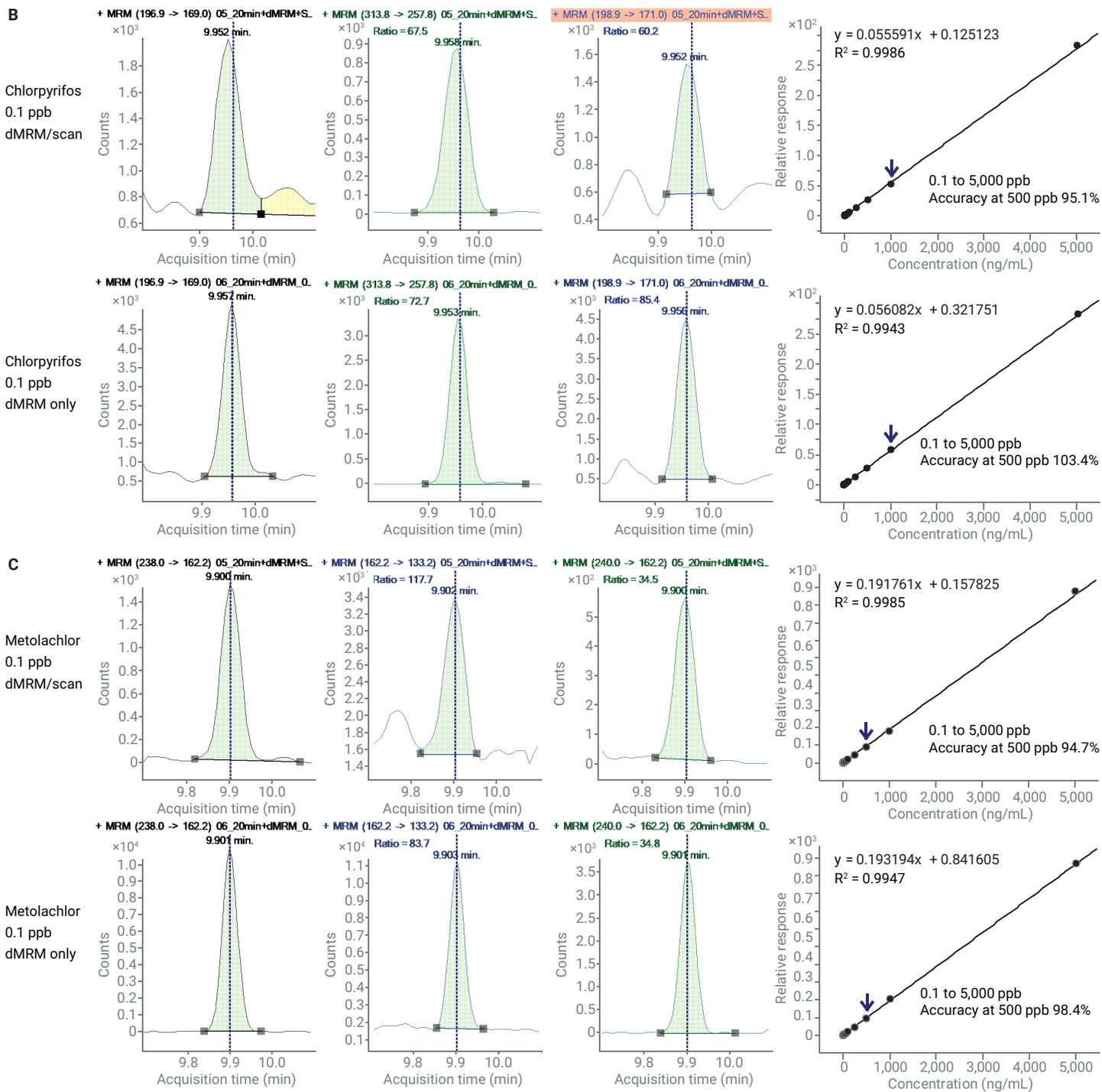
**Figure 8B,C.** Quantifier and qualifier ion profiles and matrix-matched calibration curves over 0.1 to 5,000 ppb for chlorpyrifos (B) and metolachlor (C) spiked at 100 ppb in cayenne pepper with the Agilent 7000E GC/TQ in simultaneous dMRM/scan and dMRM only data acquisition modes.
