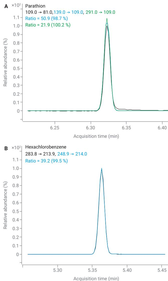
**Figure 3.** Overlays of MRM transition EICs for (A) parathion and (B) hexachlorobenzene, when using H<sub>2</sub> carrier gas and the Agilent HydroInert source on a GC/MS/MS system, showing retention of key functional groups in the presence of H<sub>2</sub>.
