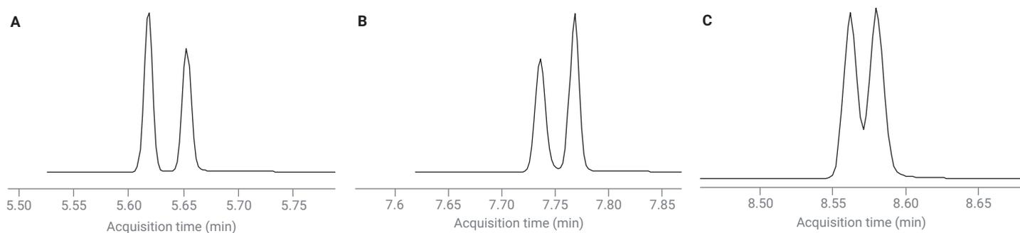
**Figure 2.** Midlevel standard (5 µg/mL) MRM transition extracted ion chromatograms (EICs) for critical isomer pairs: (A) phenanthrene and anthracene (MRM transition of 178.1 → 152.1  $m/z$ ); (B) benz[a]anthracene and chrysene (228.1 → 226.1  $m/z$ ); (C) benzo(b)fluoranthene and benzo(k)fluoranthene (252.1 → 250.1  $m/z$ ).
