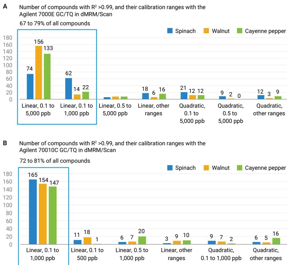
**Figure 9.** Calibration performance for the 203 pesticides with an Agilent 7000E (A) and Agilent 7010C (B) GC/TQ in spinach, walnut, and cayenne pepper QuEChERS extracts. The graph shows the number of compounds and their calibration ranges.
