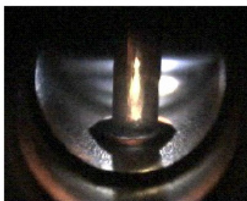
Figure 1. The view inside the tube, using the integrated camera. The probe is dispensing the sample into the tube.
