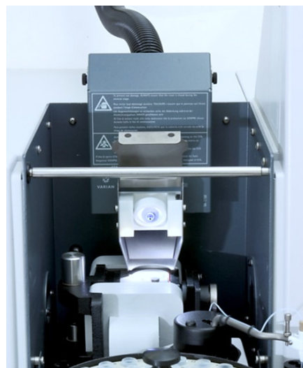
Figure 3. The optional fume extraction accessory includes an LED lighted mirror to provide a clear view of the graphite tube injection hole. Alignment of the autosampler capillary is worry-free while the exhaust system removes ashing vapors at their source. The extraction accessory provides flexibility of the furnace placement eliminating the need for direct position under the exhaust fan.
