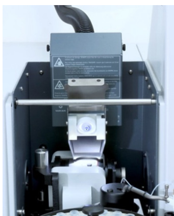
Figure 1. Agilent's optional extraction/LED accessory for the Agilent GTA 120 graphite tube atomizer.
