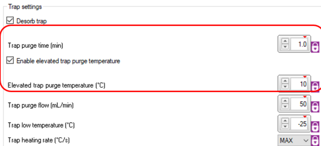
Figure 4. Enable the "elevated trap purge temperature" function in TD software.
