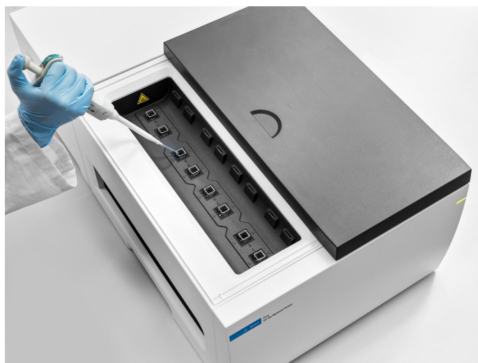
Figure 1. Agilent Cary 3500 Multicell Peltier UV-Vis spectrophotometer.
