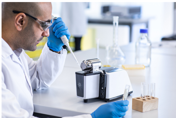
Figure 2. The liquid sample is placed onto the sample window of the Agilent DialPath module fitted to the Agilent Cary 630 FTIR spectrometer.
