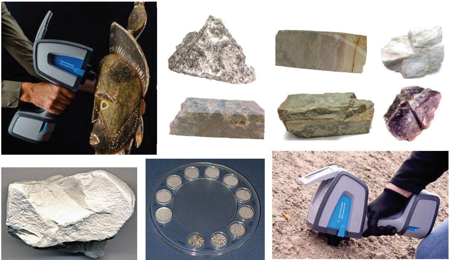
Figure 2. Examples of samples examined directly and nondestructively using the Agilent 4300 FTIR with diffuse interface in direct-DRIFTS mode. All the pictured samples have all been measured without any sample pretreatment.
