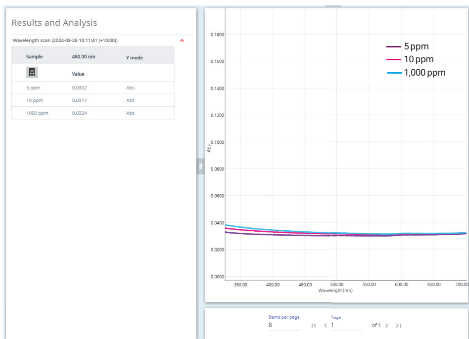
Figure 2. UV-Vis spectra of LiCl solution in water (5, 10, and 1,000 ppm) measured using an Agilent Cary 3500 Multicell UV-Vis spectrophotometer. The samples were baseline-corrected against air.
