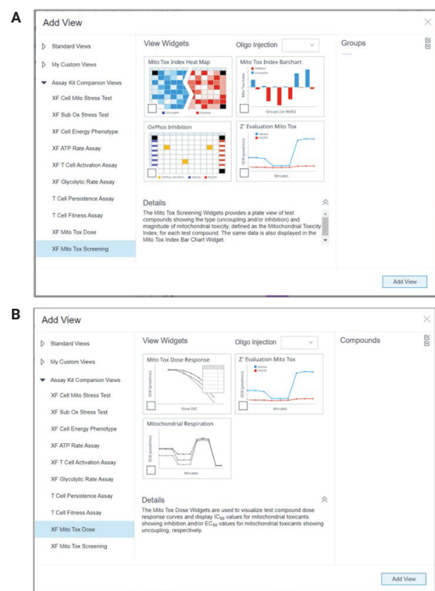
Figure 5. Agilent Seahorse Analytics Mito Tox assay companion views. (A) XF Mito Tox Screening widgets, including an MTI heat map and bar chart, an OPI detection heat map, and Z' evaluation of assay performance. (B) XF Mito Tox Dose widgets, including dose-response curves with IC_{50} and EC_{50} values, kinetic mitochondrial respiration (OCR) graphs, and Z' evaluation of assay performance.
