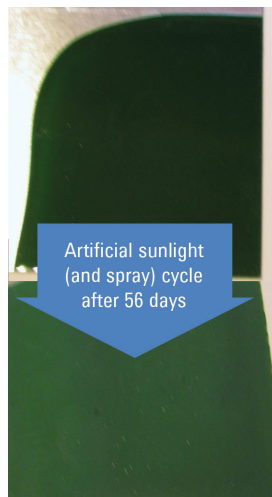
Figure 2. Two-part industrial epoxy resin finish coating sprayed onto a Q-panel, showing the visible effects of accelerated aging in a weatherometer before (unaged, top) and after 56 days (bottom: visible pin-holing).
