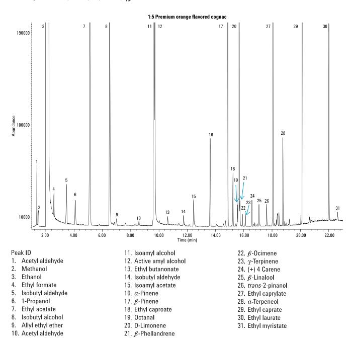
Figure 2. Total ion chromatogram of a premium orange-flavored cognac diluted 1 to 5 with distilled water in the headspace vial on an Agilent J&W DB-624UI, 30 m  $\times$  0.32 mm, 1.8  $\mu$ m column.
