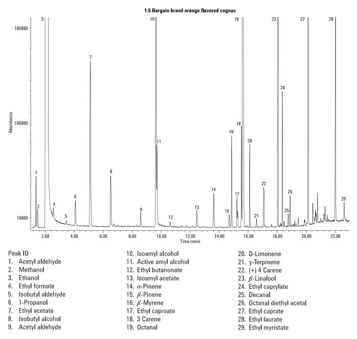
Figure 3. Total ion chromatogram of a bargain-brand orange-flavored cognac diluted 1 to 5 with distilled water in the headspace vial on an Agilent J&W DB-624UI, 30 m  $\times$  0.32 mm, 1.8  $\mu$ m column.
