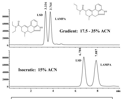
Conditions: Instrument: Agilent 1100 LC/MSD System Column: ZORBAX Eclipse XDB-C8, 2.1 x 50 mm, 5 $\mu$ m, Agilent P/N: 960967-906 Mobile Phase: as specified above, with % remaining 10 mM ammonium formate, pH 3.7 F=0.3 mL / min, Inj vol: 30 µl, Temp: 30°C, Det. MS HP 1100 MSD Conditions: SIM mode, Ions: 324.2, 223.1, 208.1 Fragmentor (dynamically ramped) 100V at 324.2, 148V at 223.1, 170V at 208.1
