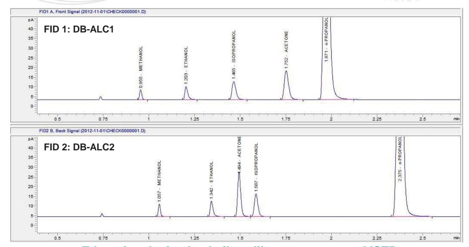
Ethanol and mixed volatile calibrator, n-propanol ISTD
