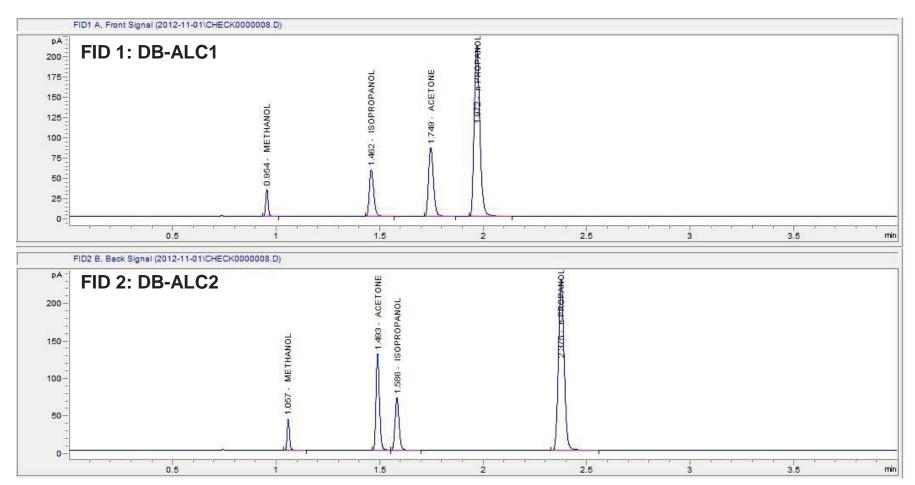
Multi-component control 0.05 % w/v per component without ethanol
